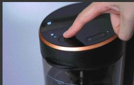
5. Pour in about 500ml clean water at 20-40°C inside. Select Water-clean mode. Clean pipe for at least 3 times until there is no residue in it.
