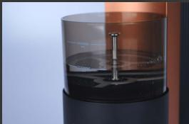
6. Clean the lower pot after elevating the platform. Wipe the bottom of the platform with a soft wet cloth.
